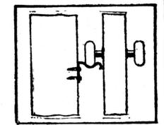
An excellent door stop can be made ed to the wall against which the door swings, and the end bent so that the doorknob fits it and prevents it from striking the wall.
