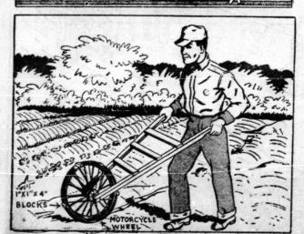
PLANT SPACER . A MOTORCYCLE WHEEL FITTED 65 MAKES A SIMPLE PLANT SPACER. BOLT OR WIRE THE BLOCKS TO THE WHEEL, SPACING THEM EQUAL DISTANCES ARABT, AND BUT WHEEL WITH TWO WOODEN HANDLES.
