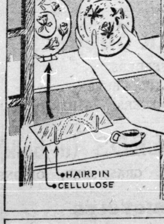
PLATE HOLDER HAIRPINS, BENT AS PICTURED, AND HELD IN PLACE WITH CELLULOSE TAPE WILL HOLD PLATES AGAINST BACK OF CUPBOARD.
