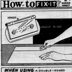
RAZOR BLADE, A HOLDER TO PROTECT FINGERS CAN BE IMPROVISED FROM A HINGE.
