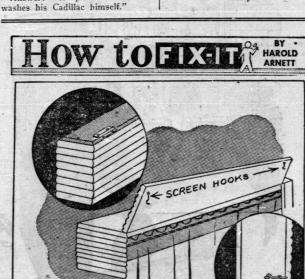
MAKE REMOVING DRAPES FROM SHALLOW CORNICES MORE CONVENIENT BY HINGING THE FACING BOARD OF THE CORNICE
