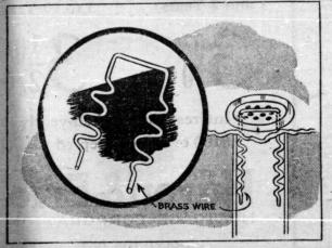
ELIMINATE NOISE OF WHIRLPOOL IN SINK DRAIN BY INSERTING LENGTH OF BRASS WIRE THROUGH HOLES IN STRAINER, BENDING ENDS AS SHOWN. TWO LENGTHS OF WIRE MAY BE REQUIRED.
