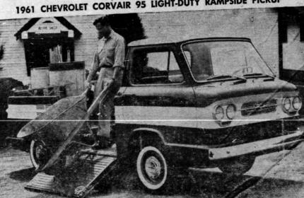
Featuring an exclusive hinged side-loading ramp, the new Chevrolet Corvair 95 rampside pickup truck offers economical operation, low loading height, easy handling, and a high proportion of cargo space to overall size. Its powered by a rear-mounted Corvair air-cooled engine designed for low operating costs. The light duty truck has a 95-inch wheel base and short overall length affording easy driving and parking in traffic or close quarters.
