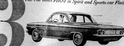
Here's what makes Corvair excitement possible. The engine is in the rear — giving outstanding traction, greater handling ease and superior weight distribution. The floor is virtually flat — whether you're seated left, right or centre there's ample room for your feet. And Corvair also features independent suspension on all wheels — so naturally the ride is smoother on any surface. But words won't replace action — so drive this peppy performer down at your Chevrolet dealer's.
