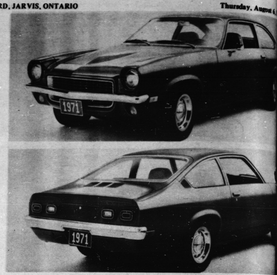
The 1971 Vega 2300 - named after the star 'Vega' - is the new little car from General Motors that "does everything well." It comes in a sturdy two-door sedan, sport hatchback coupe, slick KAMMBACK wagon and one-passenger panel express truck. The 90-horsepower engine is 2,300 cubic centimeters (140 cubic inches) with overhead valves and a die-cast, aluminum-alloy block. Compression ratio is eight to one. Lightweight and powerful, it is expected to deliver mileage comparable to any car in its class. Wheelbase is only 97 inches and overall length is 1169.7 inches, yet the Vega seats four comfortably. Shown above is the Vega 2300 Coupe.
