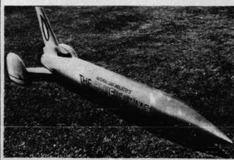
Natural gas-peroxide-fired rocket motor has the muscle to propel this uper dragster to 1,000 mph, according to its developers. It needs it two-thirds of this power to establish a new land speed record. ink what you could do with it at the stoplights
